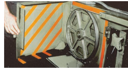
Orange 3M™ Vinyl Tape identifies dangerous machine parts that may cause injury when enclosure doors are open or guards removed.
