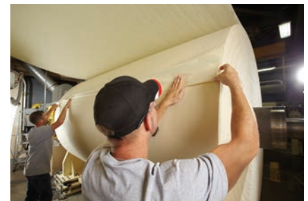
For finished mill overlap splicing, 3M™ Repulpable Permanent Tape provides high shear strength without adhesive oozing or bleed through.
