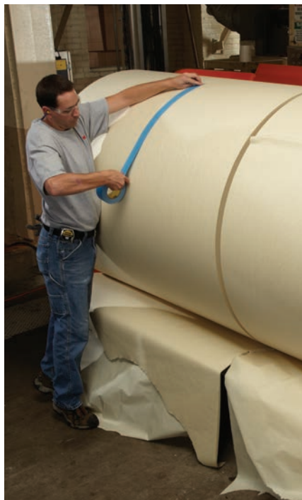
High tack 3M™ Temporary Single Coated Repulpable Tapes are available in white, blue and kraft for dependable core starting, roll closing and butt splicing.
